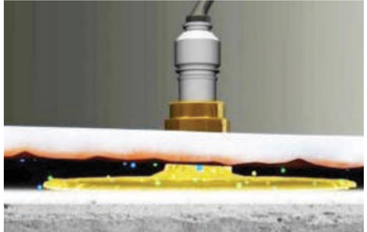
VCI Dispersion from Slurry
