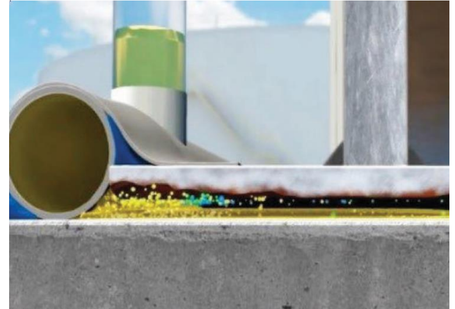
VCI Dispersion from Slurry
